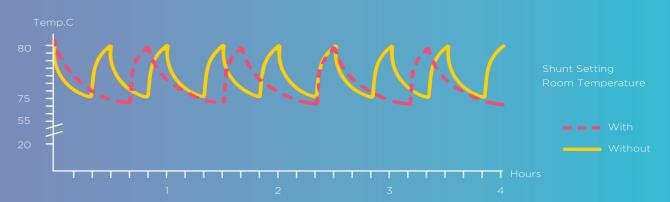
The principle is shown in the graph above where the boiler cycles across a 4 hour period are reduced from 8 to 5 and therefore the overall 'burn' time is reduced downward from 80 to 62 minutes. Reducing energy consumption by as high as 24%, in essence providing your boiler with enhanced intelligence. Glowgas complements existing building and boiler control systems, making savings possible without the need for boiler temperature or footfall adjustments.
